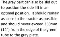
Once you have settled on a position tighten the two 12mm bolts (opposite side from image) to 90Nm (65ft-lbs)
