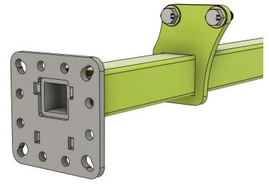
The gray plate with mounting holes is offset from the 2" tube which allows you to install it in four positions moving the attachment point a bit further forward or backwards, up or down depending on the rotation.
