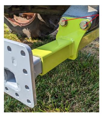
If the tractor is **NOT** equipped with a loader, then install the main green frame onto the tractor using two of the 16x40mm bolts and two of the 16mm washers as shown on the right side of the tractor as viewed from the operators seat.
