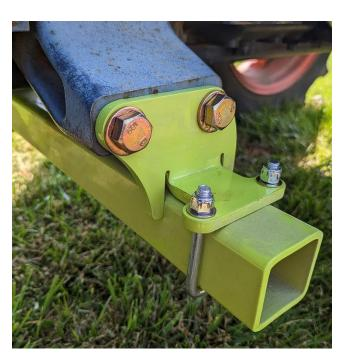
Next, install the 90degree formed green bracket as shown on the opposite (left) hand side as shown. You will need the 40mm bolts for an application with no loader and the 55mm bolts for an application with a loader(also remove the existing two bolts in the loader frame on this side).
